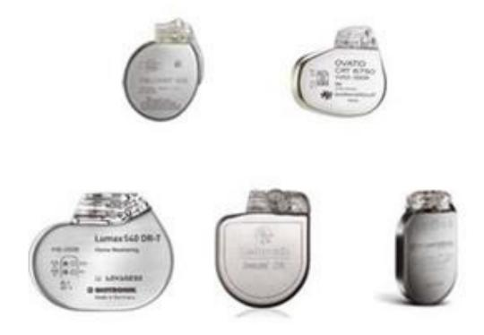
When your battery needs replacing, we replace the entire generator (see above). The wires will remain in place and will not be routinely changed.
