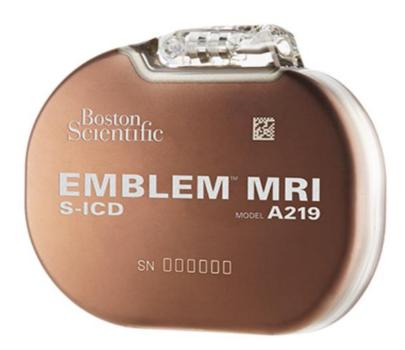
When your battery needs replacing, we replace the entire generator (see above). The wires will remain in place and will not be routinely changed.
